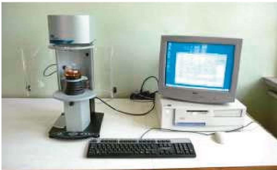
*Fig. 2. KSV Sigma 701 Tensiometer for measurements of surface tension and contact angle*
